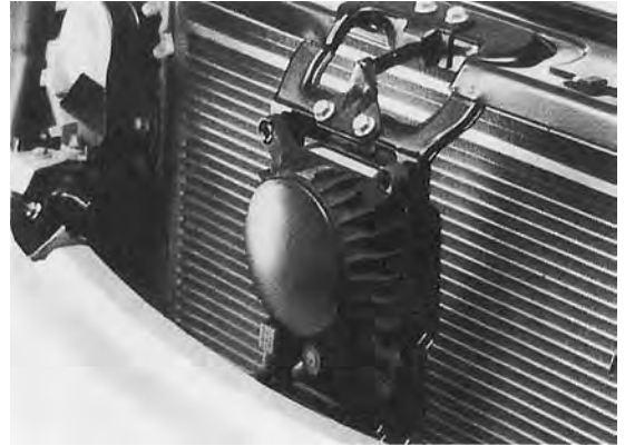
Figure 16.16 Headway sensor fitted at the front of a vehicle
