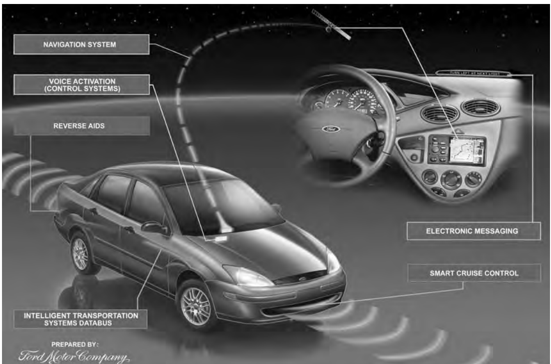
Figure 16.51 Reversing aid as part of a control system (Source: Ford)
