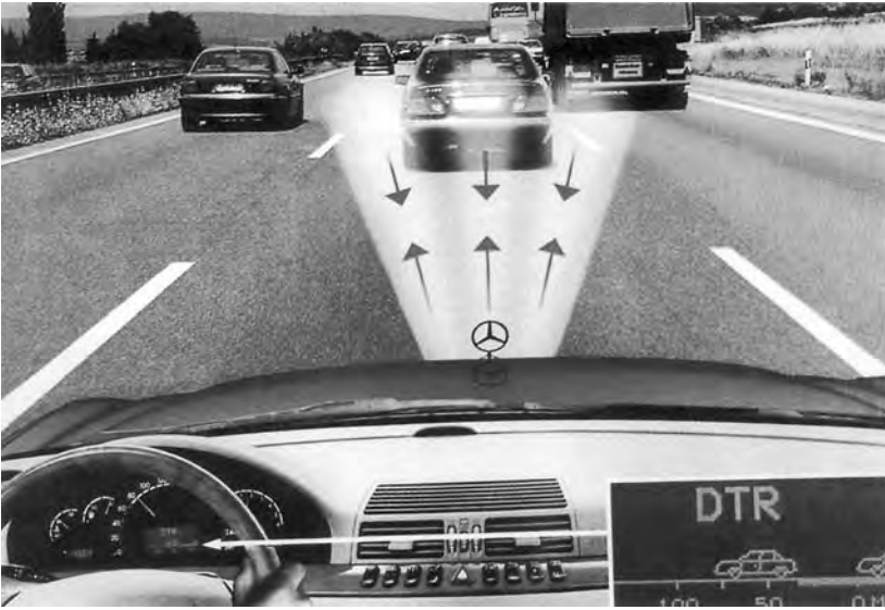
Figure 16.14 Adaptive cruise control operation
